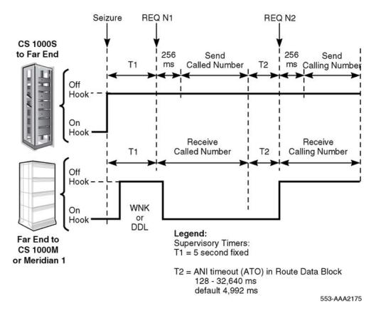
Figure 6: Supervisory signals (Bell method)
