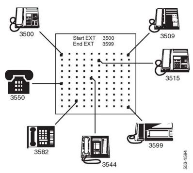
Figure 18: Enhanced Busy Lamp Field monitoring (example)
