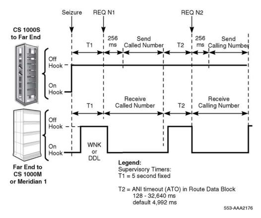
Figure 7: Supervisory signals (NT400/500 method)
